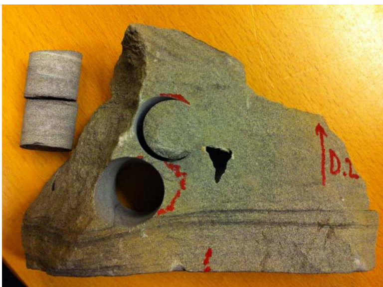
Figure 2. Sample 3 with the two plug directions and clay laminations.
